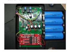
The electronics has been developed especially for our turn-table. It is a closed loop controller which keeps the speed of the motor constant. The feedback of the brushless DC-motor is compared with an extreme precise reference voltage, which makes the drive unit significant more accurate than a pll-system with quartz controlled oscillator. The outstanding feature of the TTT-Compact is the battery based power supply with LiFePo accumulators, using nano-technology. The
