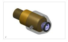
The spikes look quite common from outside, but the secret of the decoupling and leveling mechanism is inside. The spikes make the turntable standing on balls, keeping it in position by a small rubber element. This keeps horizontal vibration of the ground away efficiently. The leveling mechanism is a combination of a machined thread with a high precision sliding fit. This makes leveling of the unit easy,
